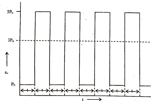
Fig: (i) Simplified load diagram of a machine under shock loading
